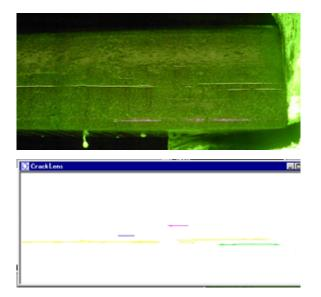
Ultra short flashes enable stung sharp images during the real time operation of the whole system. Vibrations and back-ground light don't influence the imaging process.
