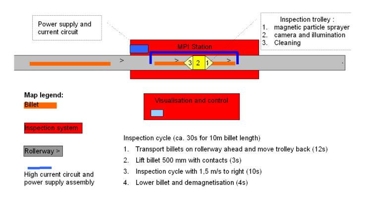
The image processing is done during camera motion. The inspection criteria can be parametrised in accordance with customer's requirements. The process monitored evaluation ensures consistent reproducible inspection quality and is fully documented.
