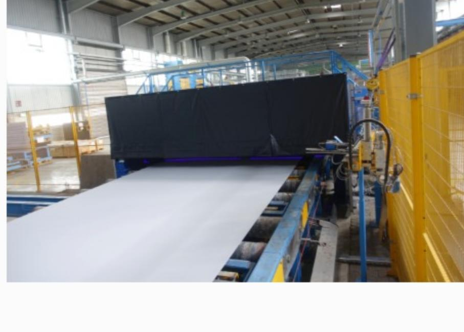
The blue laser line shows the position at which the sheet surface is scanned as it passes through. Cracks, roll-ins, shells and dents are thus detected and precisely measured.
