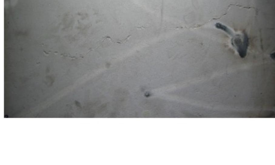
Detail photo of the sheet metal surface: The crack can be seen here by the shadow cast and by reflections on the lower edge. In addition, there are many discolorations.
